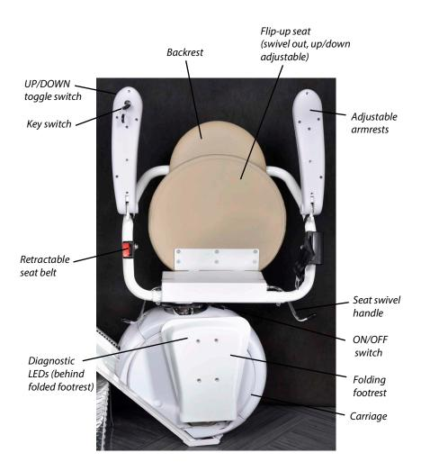
Below shows the exterior components of the K2 Stairlift (with V-seat).
